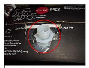
Cut off the adapter from an empty bag in box to use as a cleaning adapter
