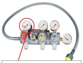
A typical contents gauge will have a red segment. Ensure the needle is near or above this zone.
